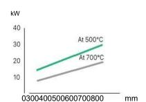
The power ratings range from 8kW to 30kW, corresponding to heating lengths from 300mm to 700mm.
