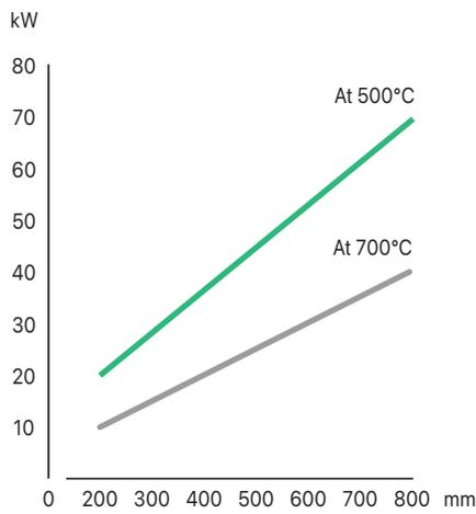
The power ratings range from 10kW to 70kW, corresponding to heating lengths from 200mm to 800mm.
